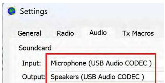
Figure 5 — A sample of what WSJT-X should look like when setting up the audio devices.
