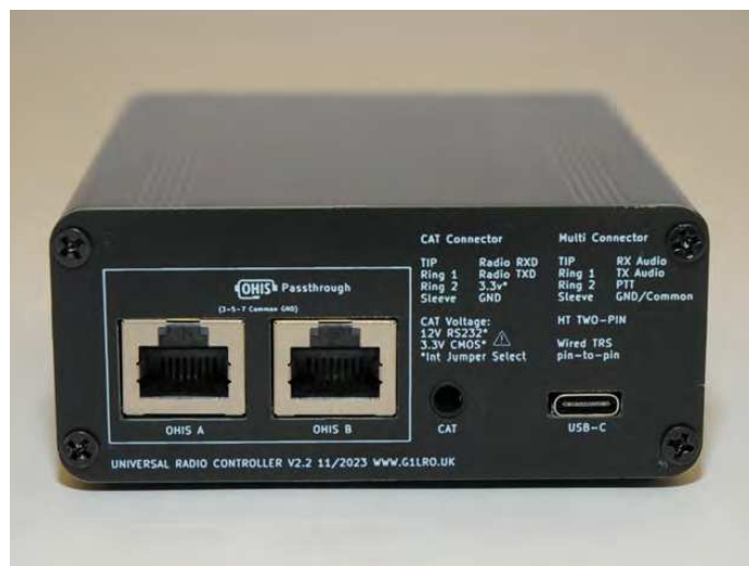
Figure 14 — The rear panel of the Halibut Electronics G1LRO Universal Radio Controller unit.
