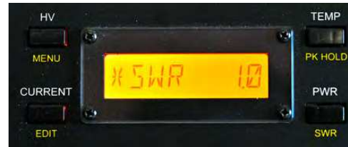
Figure 4 — A KPA500 SWR readout of a three-element 6-meter Moxy at 50.313 MHz.
