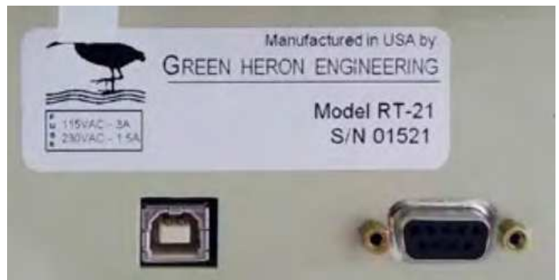
Figure 2 — The back of an Elecraft KPA1500, an Icom IC-7610, and a Green Heron RT-21 showing the USB-B port.
