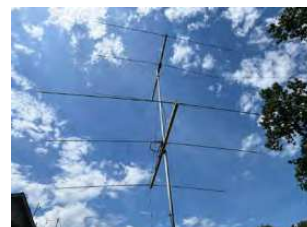
The deployed tomato stake 6-meter array.
