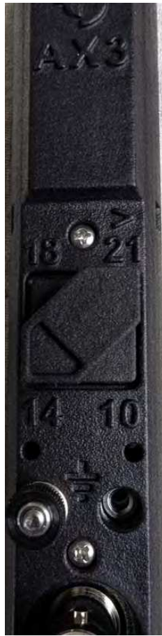
Figure 6 — The Elecraft AX3 jumper block selects 20 meters.
