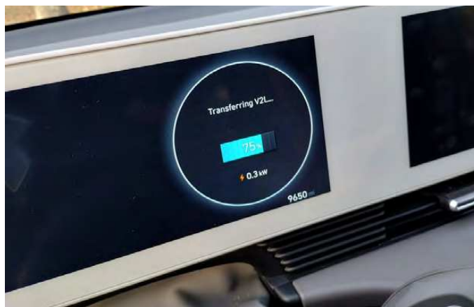
Figure 2 — The V2L display during the author's 100 W FT8 transmissions. Note that the display is 0.1 kW (100 W), and it fluctuated between 0.1 and 0.3 kW during transmit. [Rob Suggs, NN4NT, photo]
