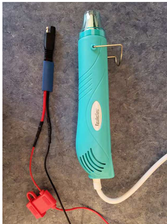
Figure 4 — An embossing heat tool, which can be useful for projects involving solder paste or heat-shrink tubing. [Jody Nelis, K3JZD, photo]
