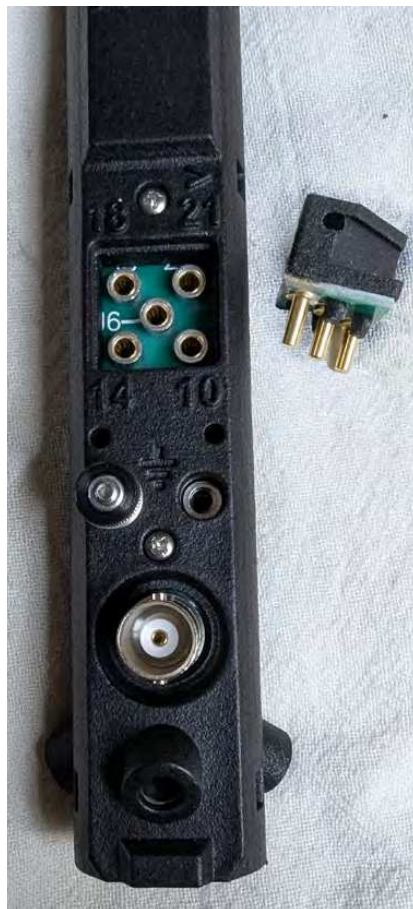
Figure 5 — The Elecraft AX3 band change socket and jumper block.
