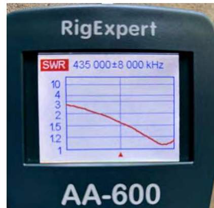
Figure 5 — The SWR with shorter quad loops. Making the loops longer will lower the resonant frequency. [Richard Lawn, W2JAZ, photo]
