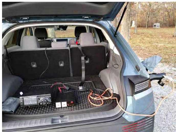
Figure 1 — The author's POTA setup at Chickamauga and Chattanooga National Military Park (US-0716), which includes a Yaesu FTDX10 and a Samlex power supply connected to his Hyundai IONIQ 5's V2L port. The USB cable runs to the back seat, where his laptop is set up. [Rob Suggs, NN4NT, photo]
