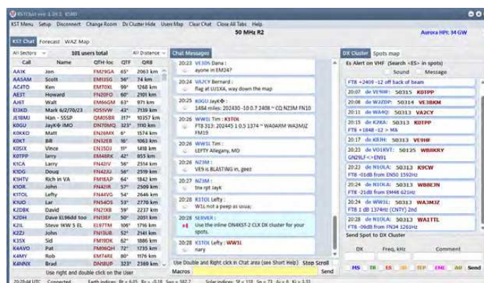
Figure 2 — KSTChat is another option for scheduling meteor-scatter contacts. This software pulls information from the ON4KST amateur radio chat room.
