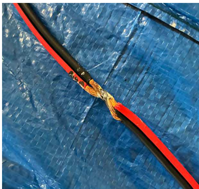
Figure 5 — A photo of the gamma tee match.
