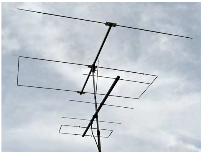
Figure 1 — Dave Ahlgren’s, K1BUK, 6- and 2-meter Moxy antennas on a 16-foot painter’s pole.
