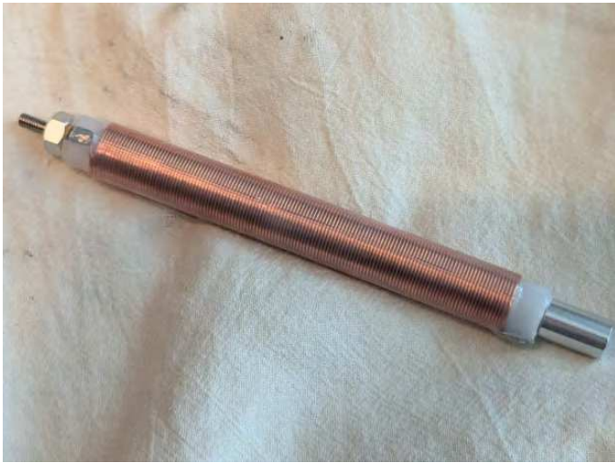
Figure 4 — The Elecraft AXE1 40-meter extender coil.
