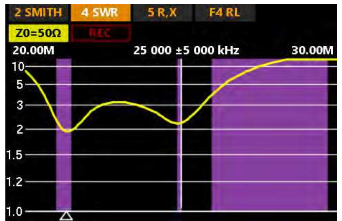
Figure 12 — The Elecraft AX3 15-, 12-, and 10-meter SWR sweep.
