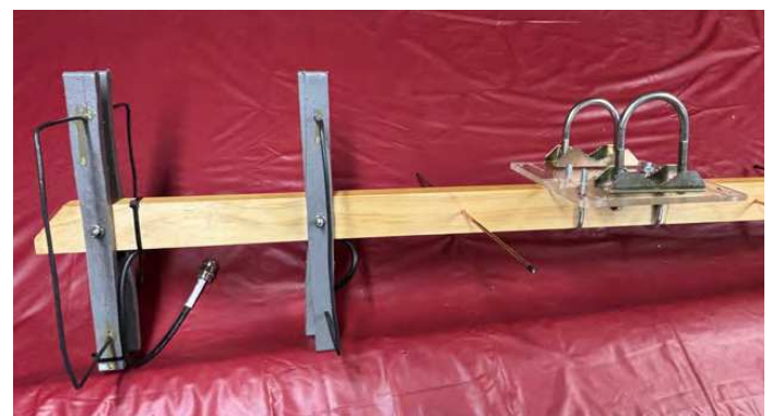
Figure 3 — The Quagi with a cross-boom mount. [Richard Lawn, W2JAZ, photo]
