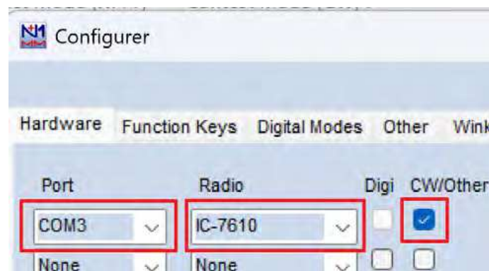
Figure 6 — A sample of what N1MM should look like when connecting it to the IC-7610.
