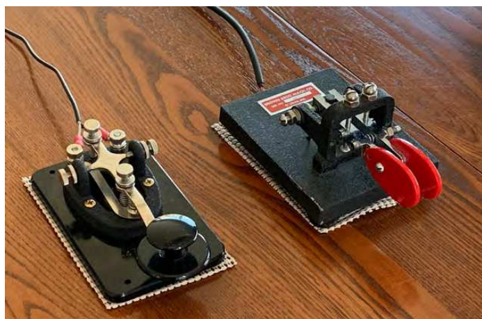
Figure 3 — A Johnson Speed-X hand key (left) and a Brown Bros iambic key (right), both held in place via shelf liner. [Scott Freeberg, WA9WFA, photo]
